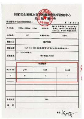
The sound insulation and noise reduction performance of vacuum insulated glass is based on the fact that sound does not propagate in vacuum chamber. The Weighted Sound Reduction Index at full frequency band can reach up to 39dB ( CTC National Inspection Group Report ), while the weighted sound reduction index of regular insulated glass is 28 dB.
